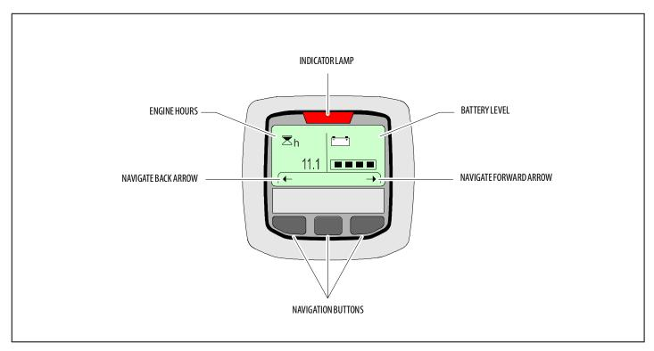
Figure 3-6. Ground Control Console Display Gauge
