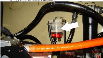
Lube Point(s) - Replaceable Element Interval - Drain water daily; Change every year or 600 hours of operation
