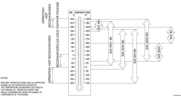
ENGINE OIL OR OPERATION OUTSIDE OF THE TEMPERATURE BOUNDARIES OUTLINED IN THE "ENGINE OIL OPERATION CHART" MAY RESULT IN PREMATURE WEAR OR DAMAGE TO COMPONENTS OF THE ENGINE.
