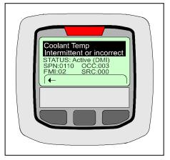
Figure 3-5. Engine Diagnostic Screen
