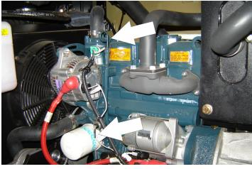
Lube Point(s) - Fill Cap/Spin-on Element Capacity - 6 qt. (5.7 L) w/filter
