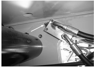
Figure 2-5. Tower Boom Vertical Limit Switch
