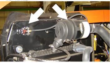
Lube Point(s) - Replaceable Element Interval - Every 6 months or 300 hours of operation or as indicated by the condition indicator
