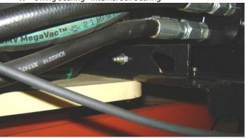
Lube Point(s) - 2 Grease Fittings Capacity - A/R
