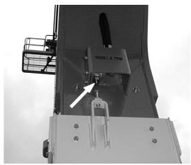
Figure 2-6. Tower Boom Horizontal Limit Switch
