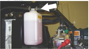
Lube Point(s) - Fill Cap Lube - Anti-Freeze Coolant (Refer to Engine Manual for compatible coolants) Capacity - 6 qt. (5.7 L)
