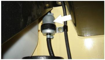
Lube Point(s) - Replaceable Element Interval - Change every year or 600 hours of operation
