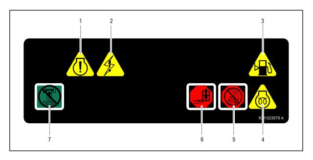
Engine Malfunction/Check Engine 4. Glow Plug
