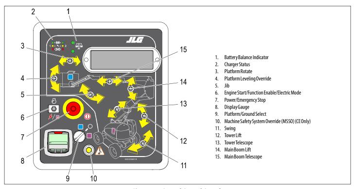
Figure 3-1. Ground Control Console
