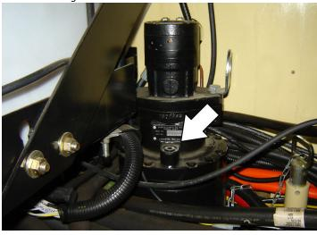
Capacity - 43 oz. (1.3 L) Lube - 90w80 Gear Oil Interval - Check level every 3 months or 150 hrs of operation; change every 2 years or 1200 hours of operation
